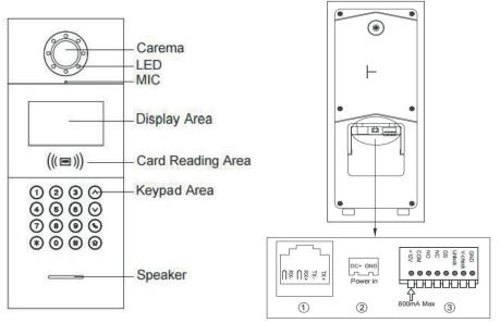
Network Interface (Non-standard PoE 24V power supply; if power is needed for gate lock or low temperature heating function is required, outdoor station must be supplied independently).)
